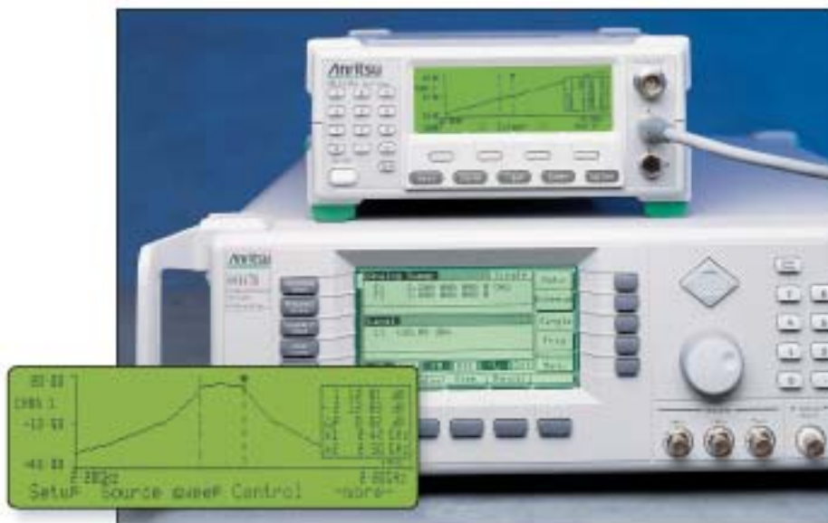
Source Sweep Graphic Display. Acquire power sweep or frequency sweep data at speeds greater than fifteen sweeps per second ( GPIB to PC screen update rate). The meter automatically generates sweep synchronization with Anritsu 68000B or 69000A series Synthesized Sweep Generators.
