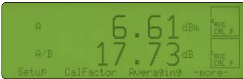
True dual channel display shows amplifier output power and gain simultaneously
